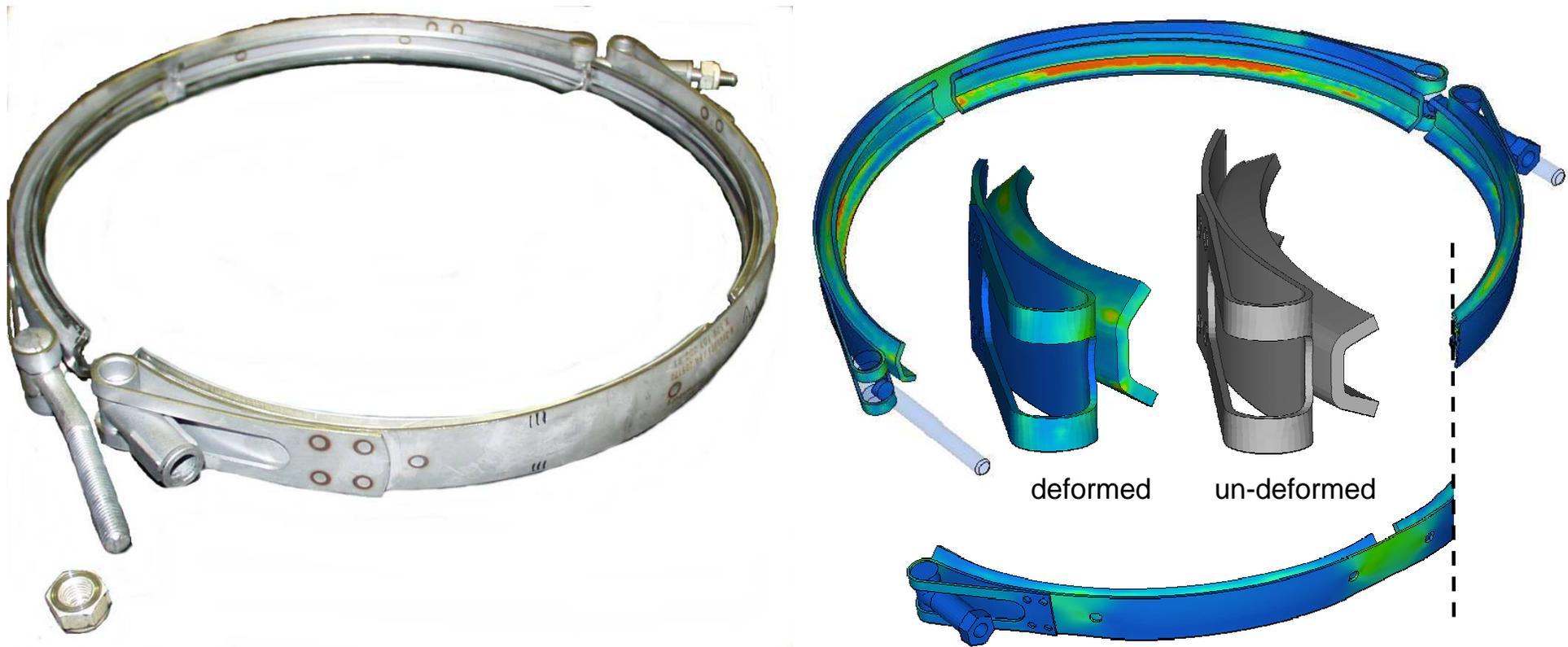
significant plastic deformation of v-shaped lower strap
