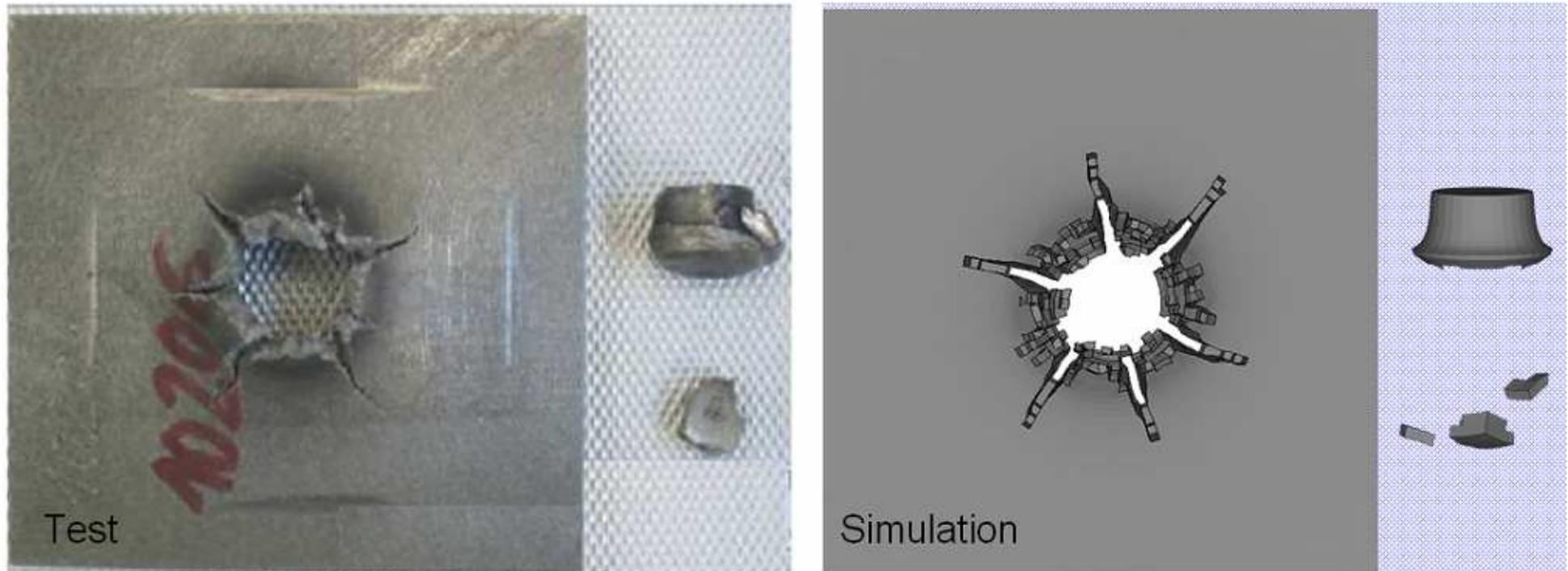
The **optimised** material law with the enhanced material and the additional failure specification leads to an excellent correlation of deformation and failure behaviour and meets the specific energy which is needed for a full penetration
